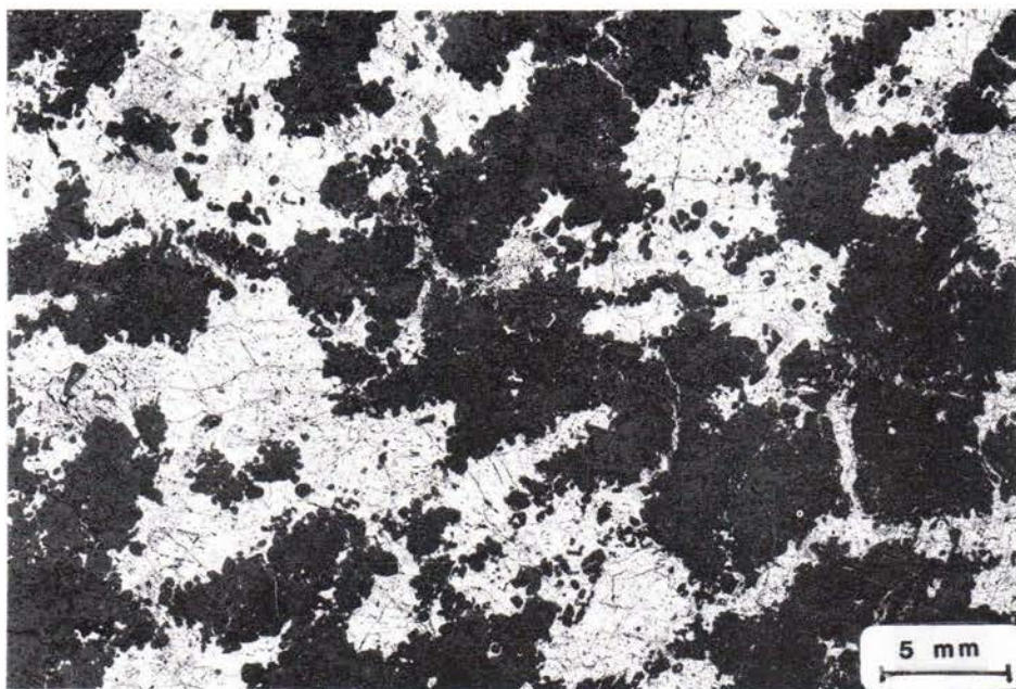
Fig. 31. Oriented dissemination (buck shot ore) with interstitial margins. Oravainen, Ni ultramafite. Photo E. Halme.
