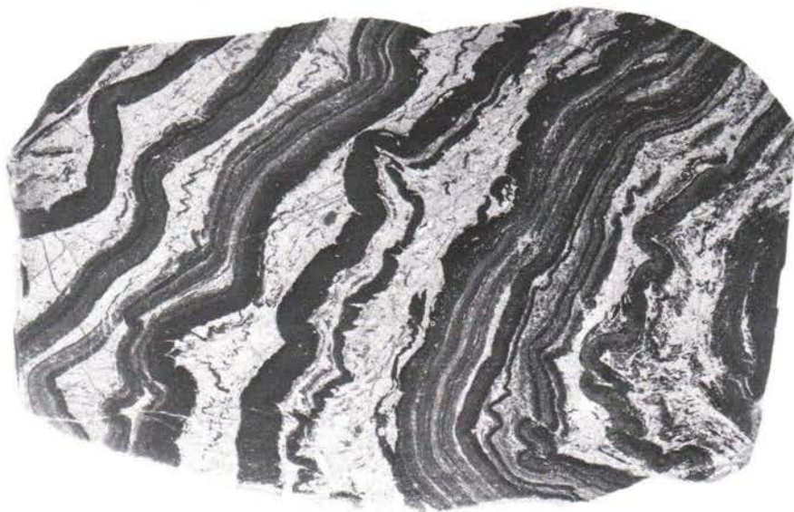
Fig. 15. Ni-Cu ore types of the Pechenga deposits. a — high-grade dissemination in serpentinite; b — breccia ore, c — massive ore; d — mineralized phyllites.
