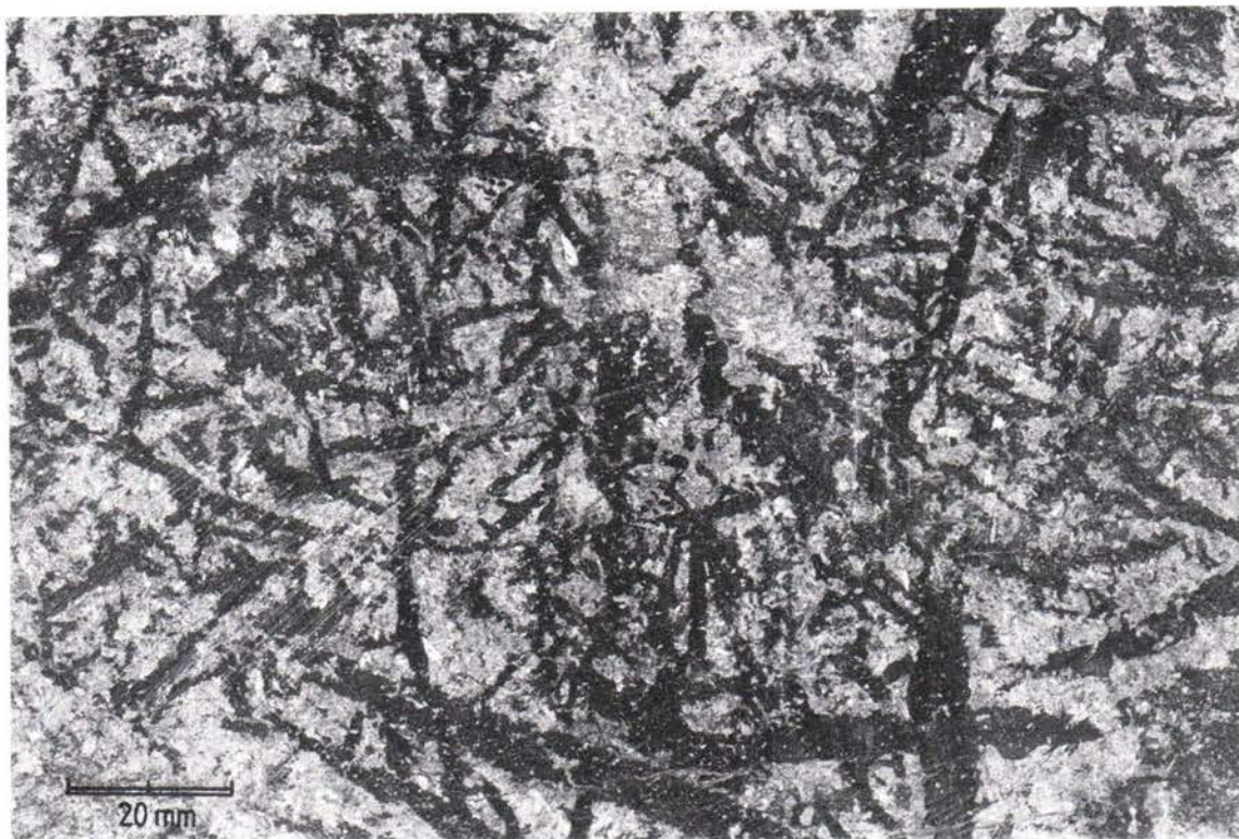
Fig. 13. »Jackstraw-texture» in metaperidotite from the Lappvattnet deposit. Polished surface.
